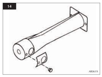
9.5 Reassemble in reverse order with correct aeration plate(s). NOTE: EVEN IF NO AERATION PLATE IS REQUIRED, THE SMALL SCREW(S) MUST BE REPLACED.
